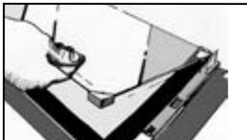
This assembly comprises 2 glass windows, the 1<sup>st</sup> of which has 2 rubber stops on the 2 front corners.
