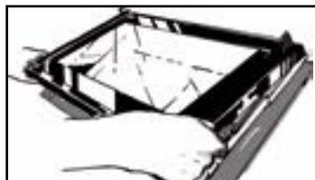
Make sure you correctly slot the frame under the spigot next to the hinge.
