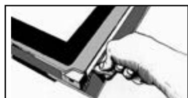
Lever the assembly to detach the frame and the glass. Conduct the same operation on the left.
