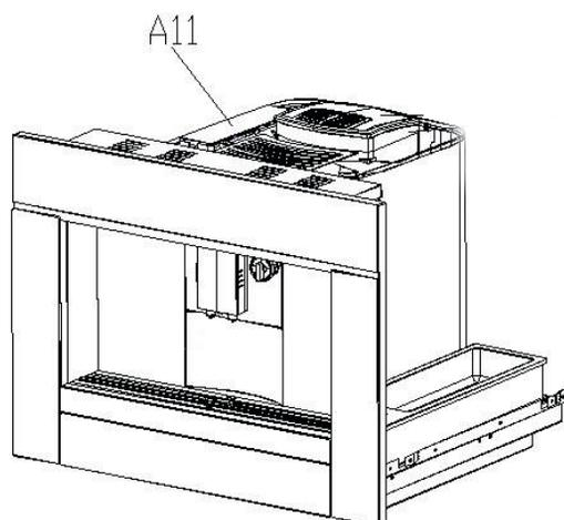
Step 6: open the tank cover in left side A11.
