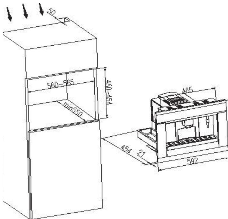
Step 1: install guide connect bracket – fix with the screws if use side install method.
