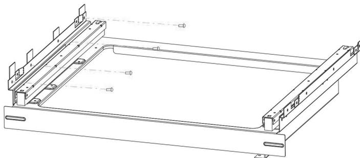
Step 2: fix with the screws. If use button install method.
