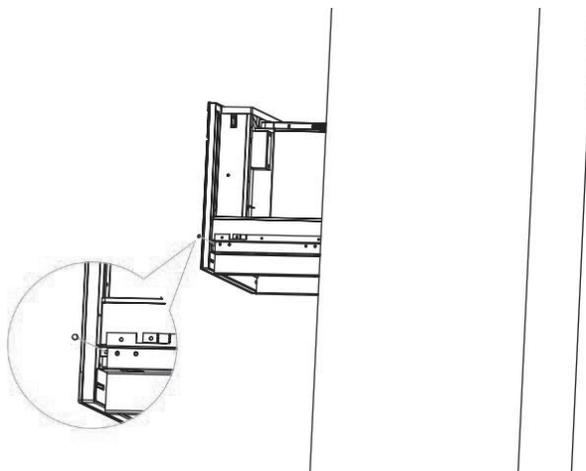
Step 5: Extracted this machine to outside. Open the coffee bean cover to add coffee beans in container.
