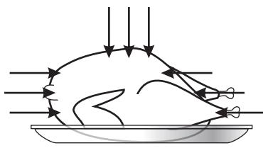
The friction between molecules produces heat which raises the temperature of the food, de-freezing it, cooking it or keeping it hot.
