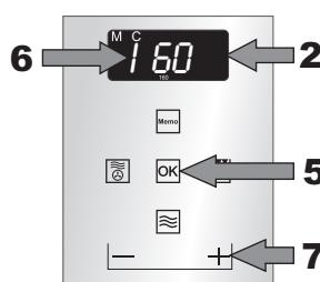
The display **2** shows a temperature **6**, in our example 160 °C. The temperature could be changed.
