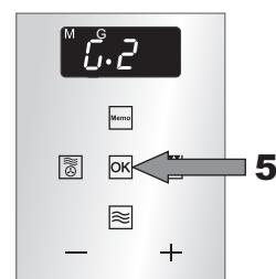
The display **2** shows a symbol **3**, **G** to display a kind of operating function and a symbol **4**, **G.** to display it's variant.
