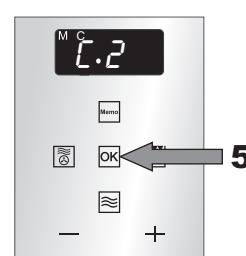
The display **2** shows a symbol **3**, **C** to display a kind of operating function and a symbol **4**, **C.** to display its variant.
