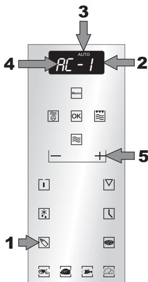
The oven has default cooking menu for simple operation. Touch the key to select desired auto cooking function. Choose the appropriate function according to the food type and weight.
