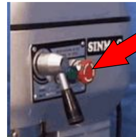
Picture 1. Emergency stop button. A red mushroom safety switch. Push in to stop the machine. Twist and pull out to reset.
