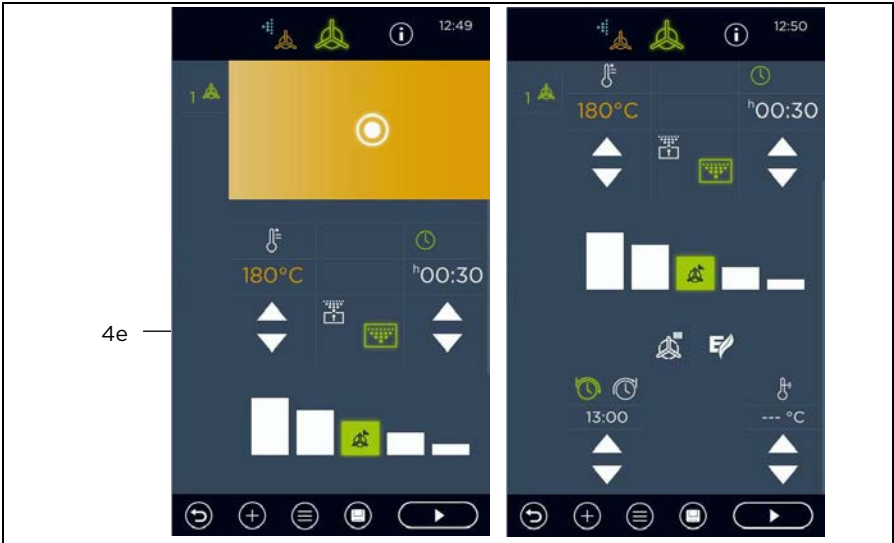
Fig. 61: Manual baking screen in baking operating mode without steam injection (Climatic® MT monitor displayed and hidden)
