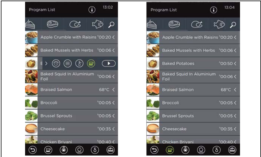
Fig. 46: Selection of Multi Cooking in the action line of a program (left) or in the special program line (right)
