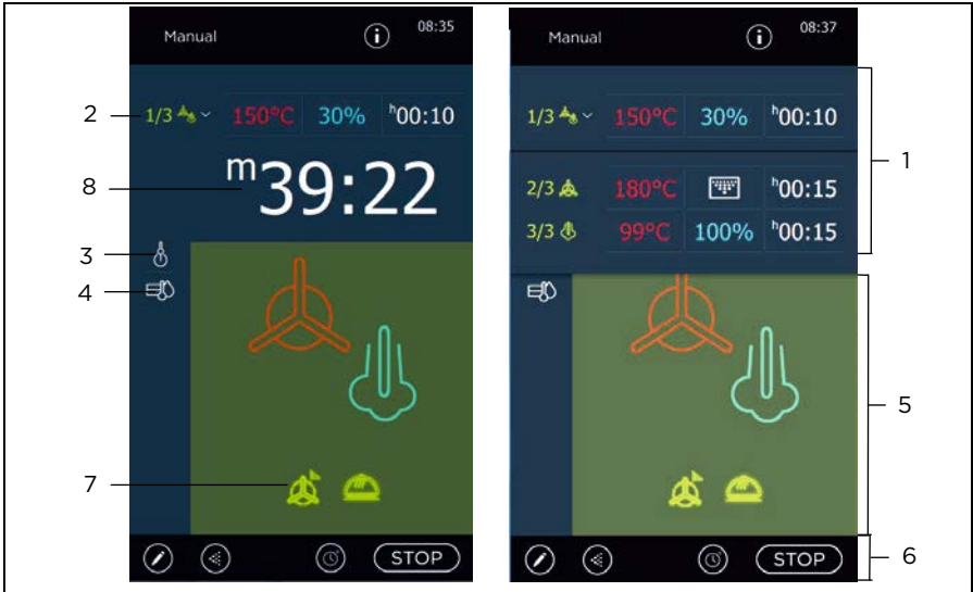
Fig. 53: Ongoing operation screen for the cooking program (closed step display, left and open step display, right)
