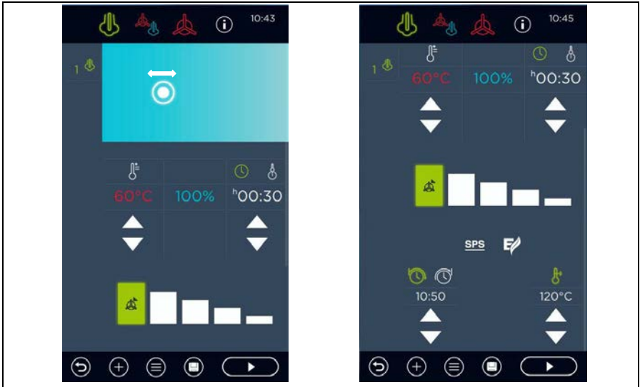
Fig. 21: Manual cooking screens for steam mode (Climatic® MT monitor displayed and hidden)
