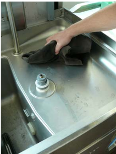
Wipe with a cloth the tank and check for any debris on the bottom.
