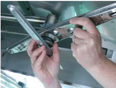
Keeping with a hand the washing arm in place, screw the rinse arm.
