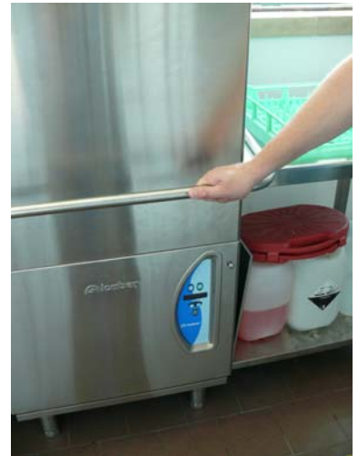
Completely close the hood the dishwasher. If there is an extended downtime, it is advisable to leave the hood open.
