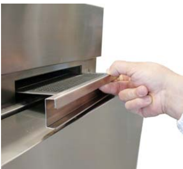
(only for L305-CV) Clean the filter of the steam condenser that is placed in the upper part of the hood;
