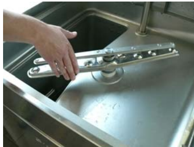
Check that the wash and rinse arms are free to rotate (upper and lower)
