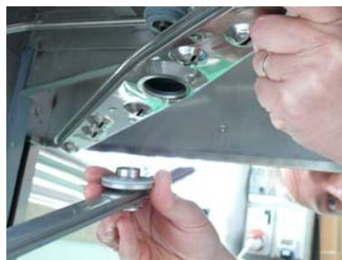
Remove the reel clearing top
