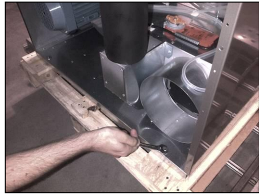
-UNSCREW WITH A FLAT SPANNER NO. 13
