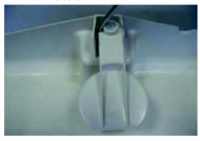
Check nozzle orifice condition. In case of obstruction clean it by pin
