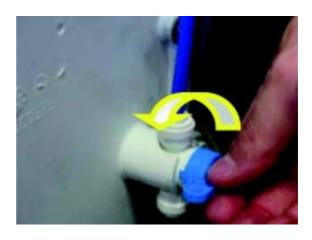
Bend down the plastic hose and drain out rthe water from the water sump than move it up again.
