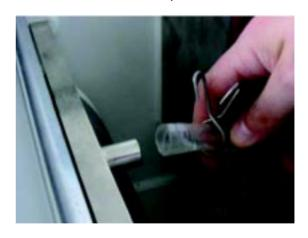
Lift the water pump up to release it from sliding holding screw
