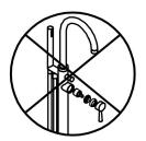
Caution: Do not disassemble the main valve core components without permission
