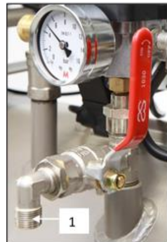
Fig. 14: Connecting to the compressed air outlet
