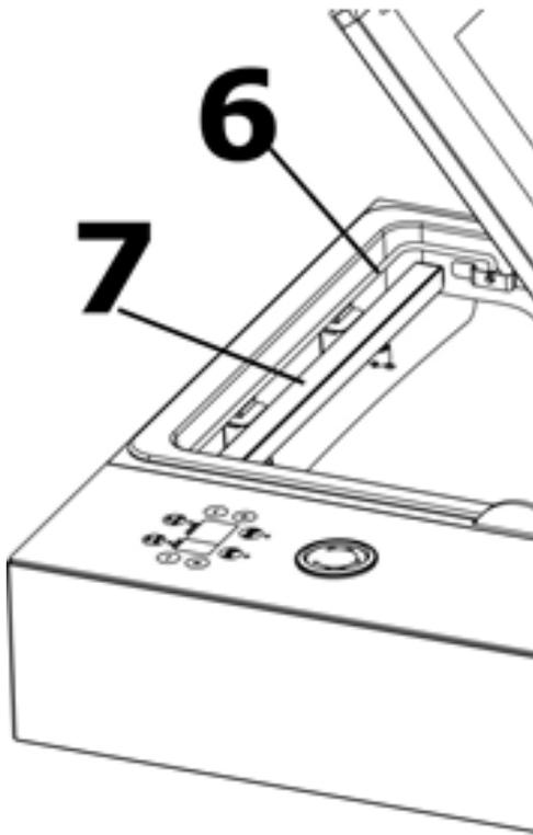
6 Fixation: Fix the bag during vacuum and sealing. Lift and clamp down to fix the bag.
